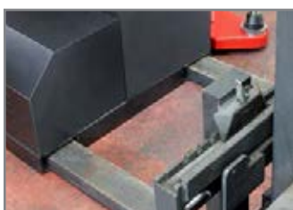
INFORCAMENTO POSTERIORE MACCHINA BACK HOLES FOR MACHINE FORKLIFTING
